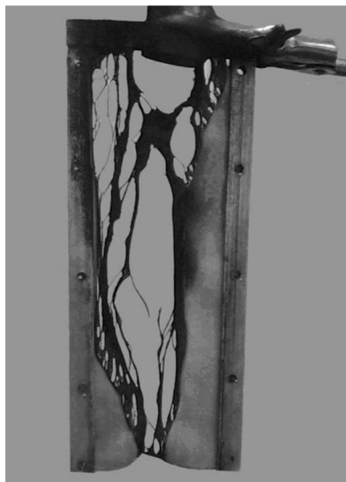
FIGURE 1 Mostashari's flammability tester with low add-ons applied onto a polyester fabric after the end of the experiment. Uneven burned and carbonaceous areas in the fabric are illustrated in the figure.
